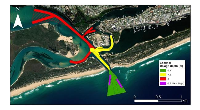
Figure 7: GLOA navigational channels and design depths
