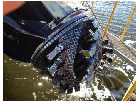
Figure 50: Cutter suction head on Dredger Kalimna
