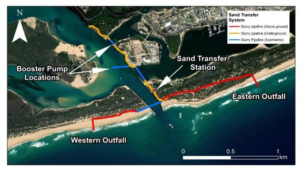
Figure 51: Sand Transfer System infrastructure locations
