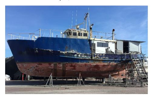
The ex-commercial vessel has been partially converted to a liveaboard and has some building materials and parts on board. The engine is a Detroit 8V91 318hp 2-stroke diesel with an Allison hydraulic transmission and Onan generator. Machinery and fittings on board are in fair condition and could be salvaged and repurposed.
