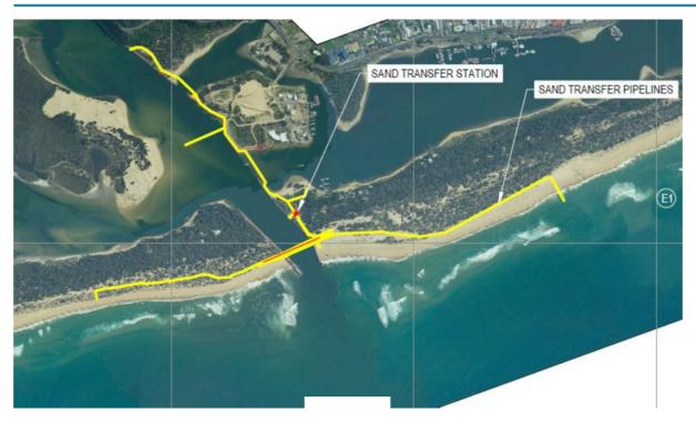
Figure 6: Layout of the Sand Transfer System
