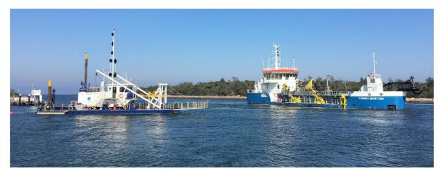
Figure 2: Kalimna CSD and Tommy Norton TSHD operating in the Inner Channels
