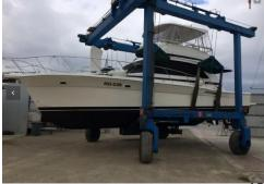
Mallacoota slipway (16 tonne capacity) is located adjacent to the main boat ramps. Gippsland Ports undertakes slippings and launchings. Once a vessel is slipped, maintenance work is carried out by the owner, contractors and or support personnel.
