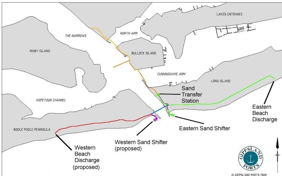
**Figure 2: Elements of the Sand Transfer System**
